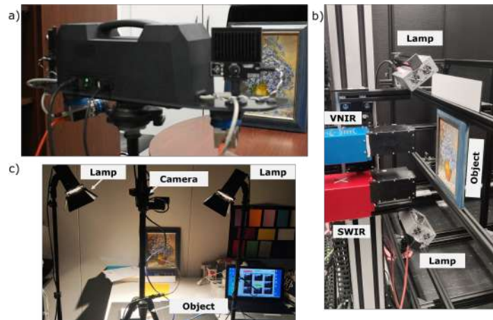
Figure 5.22: The systems used for reflectivity measurements: a) MIS, b) HySpex c) SpectroCam.
